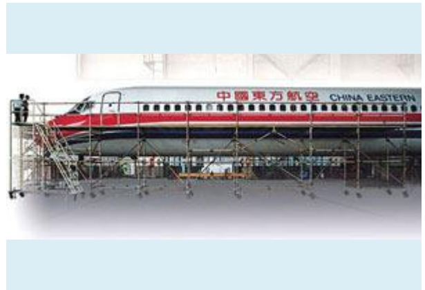
Re-assembly fuselage platform
